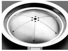
Continental's Preformed Composite Rupture Discs also feature our sevenhole pattern, positioned at the apex of the rupture disc's top section. This unique configuration, in combination with the pre-cut sections along the dome, provide non-fragmenting characteristics when used with a non-metallic or TEFLON®\*\* seal. By using this sevenhole design, thicker, more durable materials can be used to manufacture the rupture disc while still achieving the high 80% operating-to-burst-pressure ratio.
