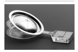
The CDC Type Rupture Disc is the basic Preformed Composite Rupture Disc design consisting of a slotted metallic top section and a TEFLON or metallic seal on the top section's process side. This basic design provides corrosion protection and excellent performance in low pressure applications where no backpressure or vacuum is expected.
