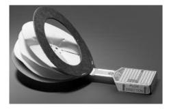
The ENVIRO-SEAL Type I Rupture Disc is designed to burst in only one direction. The rupture disc consists of a single metallic top section located on the vent side of the rupture disc with a single non-metallic seal located on the process side of the rupture disc. The ENVIRO-SEAL Type I Rupture Disc provides excellent protection and corrosion resistance for applications requiring single direction overpressure protection.
