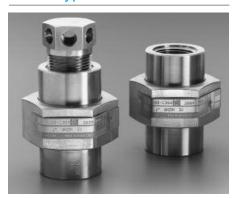
C.D.C.'s Union Type Holders are designed for piping connections using 1/2", 1", 1-1/2", and 2" (13mm, 25mm, 40mm and 50mm) size piping. All Union Type Holders are available with threaded or welded inlets in combination with threaded, welded, or muffled outlets. Available materials include Carbon Steel and 300 Series Stainless Steel. Special designs are available upon request. Refer to C.D.C. Bulletin 2-3308-2 for details.
