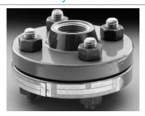
The Full Bolted Style Holder is available for ANSI, DIN, or JIS class flanges. Full Bolted holders for Preformed Composite Rupture Discs are available in sizes ranging from 1" through 24" (25mm to 600mm) in the 30° angular seating configuration. Standard materials include Carbon Steel and 304 or 316 Stainless Steel. Special materials are available upon request. For additional information on other sizes or flange classes, please consult the factory.
