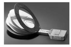
The ENVIRO-SEAL Type I Rupture Disc is designed to burst in only one direction. The rupture disc consists of a single metallic top section located on the vent side of the rupture disc with a single non-metallic seal located on the process side of the rupture disc. The ENVIRO-SEAL Type I Rupture Disc provides excellent protection and corrosion resistance for applications requiring single direction overpressure protection.
