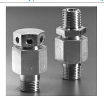
The Screw Type Holder Assembly is designed for use in "mini-systems" with pressures as high as 1000 psig (69,0 barg). The Screw Type Holder is available for a 11/16" Preformed Composite Rupture Disc and is supplied with 1/4" or 1/2" (6mm or 13mm) MPT threaded inlet and traditional MPT, free or muffled style outlets. Available holder materials include Carbon Steel and 300 Series Stainless Steel. Refer to C.D.C. Bulletin 2-2206-2 for details.
