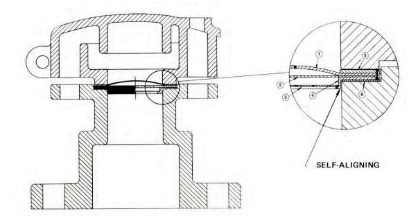
The Tanksert disc is a six (6) piece construction. The first five (5) pieces are permanently spot welded together.
