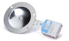
The **LOTRX®** Rupture Disc is a scored reverse acting rupture disc that utilizes failure initiating indents, a highly accurate manufacturing method to achieve and control a burst pressure at close tolerances, plus a precision semicircular score to provide a clean, consistent opening pattern.
