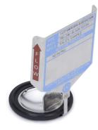
The **SANITRX HPX® II Rupture Disc** is designed to expand the SANITRX HPX® product line into higher burst pressure ratings. The geometrically strengthened arcuate on the SANITRX HPX® II provides a radiused hinge point to prevent fragmentation of the rupture disc petal upon rupture. SANITRX HPX® II also adds the 4" size rupture disc to the SANITRX HPX® Rupture Disc product family.
