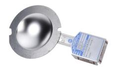
The **ULTRX® Rupture Disc** is a scored reverse acting rupture disc that utilizes failure initiating indents, a highly accurate manufacturing method to achieve and control a burst pressure at close tolerances, plus a precision semicircular score to provide a clean, consistent opening pattern.
