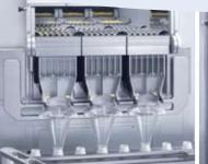
Mechanically controlled capping unit
