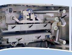
Forming station and index with integrated cooling
