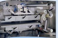
Forming station and index with integrated cooling
