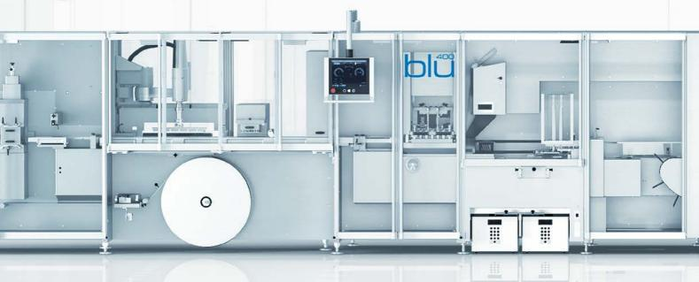
BLU 400 with LiPro feeder and punching station, plus C 2305 (overall machine length 12,898 mm)
