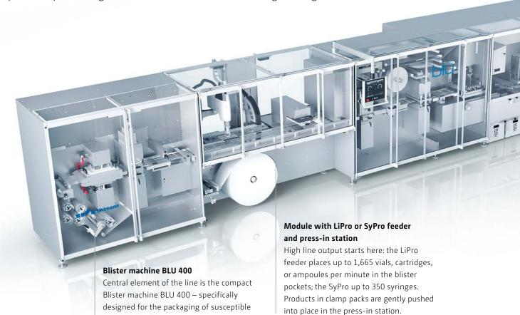
liquid dose products in clamp packs or sealed blisters. Modular in design, it attains a maximum output of 400 blisters
