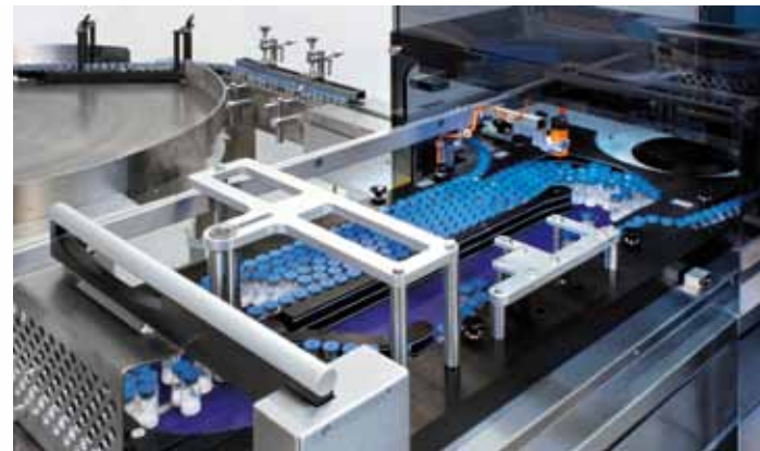
Infeed with buffer system for stable products
