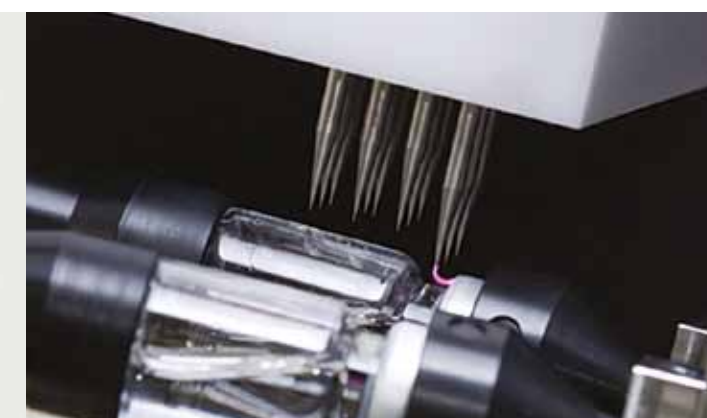
Integrated high voltage leak detection module
