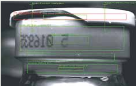
Inspection of cap, neck and stopper, optional inkjet and OCR function
