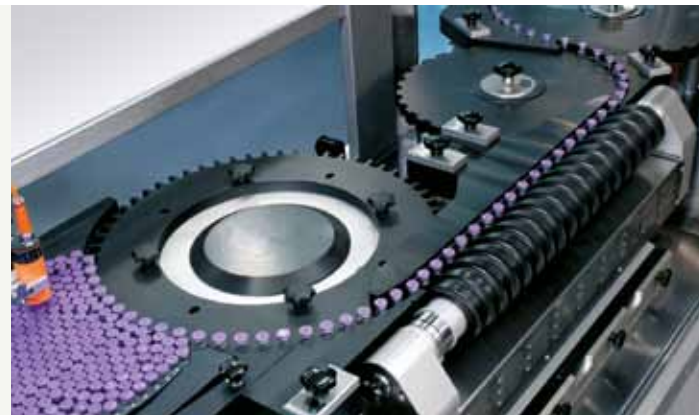
Infeed with back pressure system for instable products
