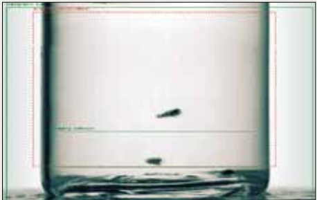
Light transmission method: Light is sent through the container side. The camera looking from the other side of the container detects shadows created by the particle.
