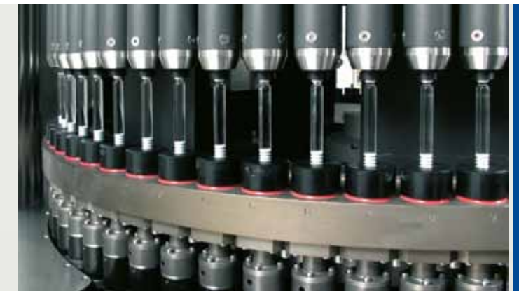
Each inspection position is equipped with programmable servo drive
