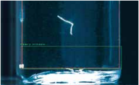
Light reflection method: Concentrated light is sent through the container bottom. The camera looking from the side detects light reflections scattered by the particle against a dark background.
