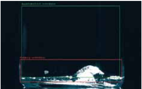
Heavy non-moving particles on the container bottom can be detected reliably by an additional window tool utilizing a special light technique.
