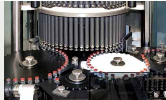
Integrated automatic re-inspection
