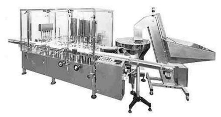
In the second half of 80's M.A.R. M50 monobloc was born to fill injectable solutions at high speed.
