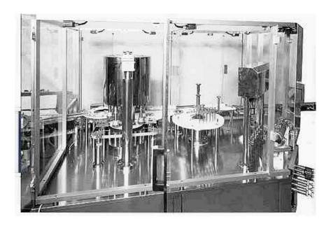
The machine can be equipped with the screw-cap application unit only or combination of different closing elements as press-on cap, etc.
