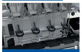
The servo driven feed screw and 'dipping' filling nozzles provide fast and accurate transportation and filling of almost any kind of bottle.
