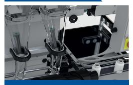
The reliable bottle reject mechanism guarantees that only correctly filled bottles are passed onto the outfeed conveyor.
