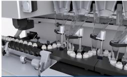
High precision feed screw and pocket wheels for fast and stable bottle transport throughout the whole filling process.
