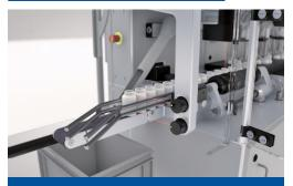
Single track bottle infeed with multiple optical sensors for verifying the presence and correct positioning and transport of bottles.
