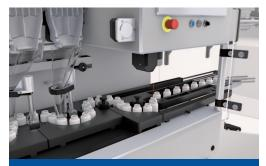
Single track output with separate reject track to remove unacceptable bottles and sample track for taking random or controlled bottle samples.
