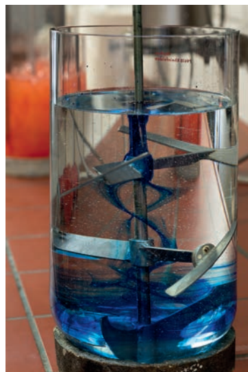
Mixing time measurement by coloring/decoloring method
