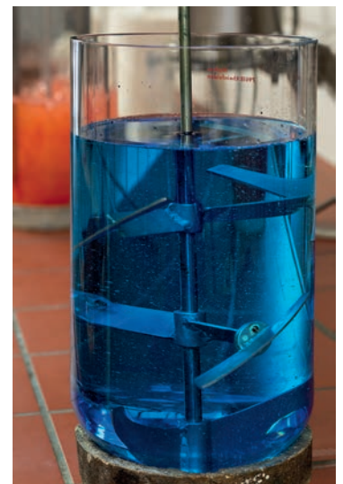
Mixing time measurement by coloring/decoloring method
